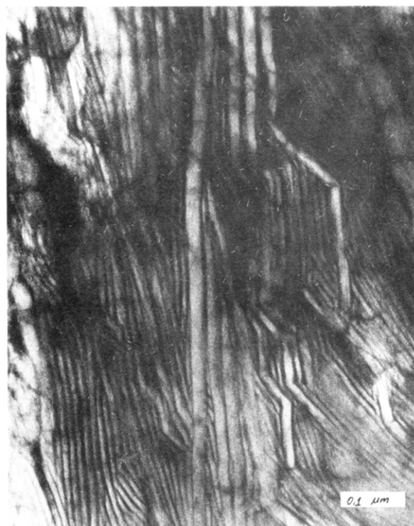
Figure 14. Transmission electron micrograph of fraction M_n = 5.6 \times 10^3 crystallized at 125 °C.
