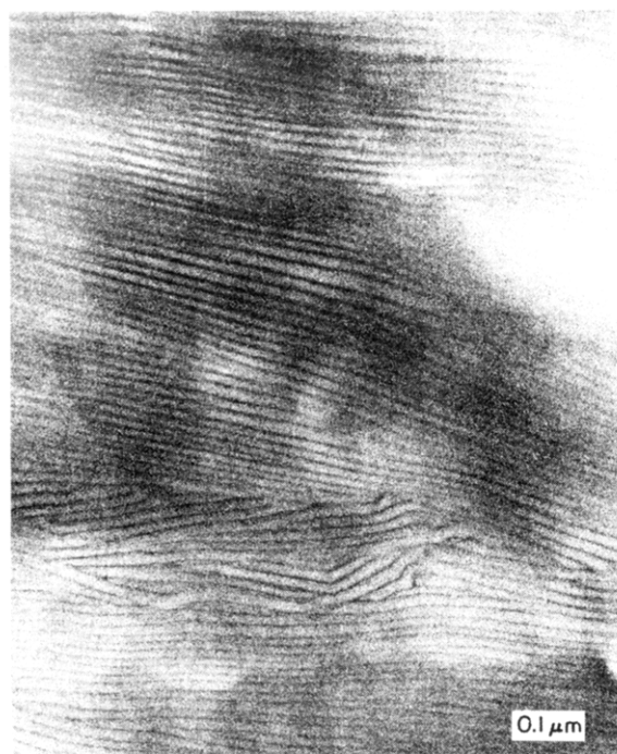
Figure 13. Transmission electron micrograph of fraction M_n = 5.6 \times 10^3 crystallized at 123 °C.
